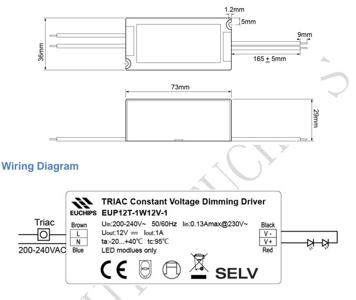
Note: For capacitive load, the larger inrush current will reduce the service life of the electrolytic capacitor.Before using this product, please contact the relevant technical personnel to match and verify.
