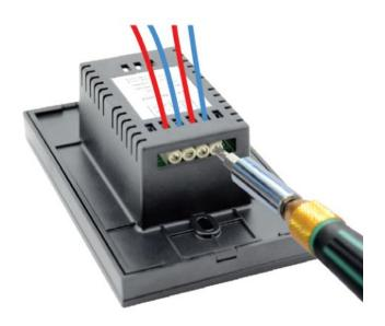
2. Gently pry gaps in touch panel with a screwdriver, and then you can slowly remove the panel, as shown below:
