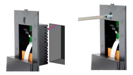
4. Buckle the glass panel to the bottom box in the right direction.
